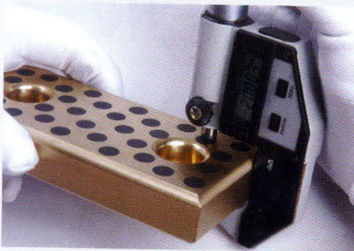
壁厚数显千分尺检测厚度 Check thickness by micrometer
